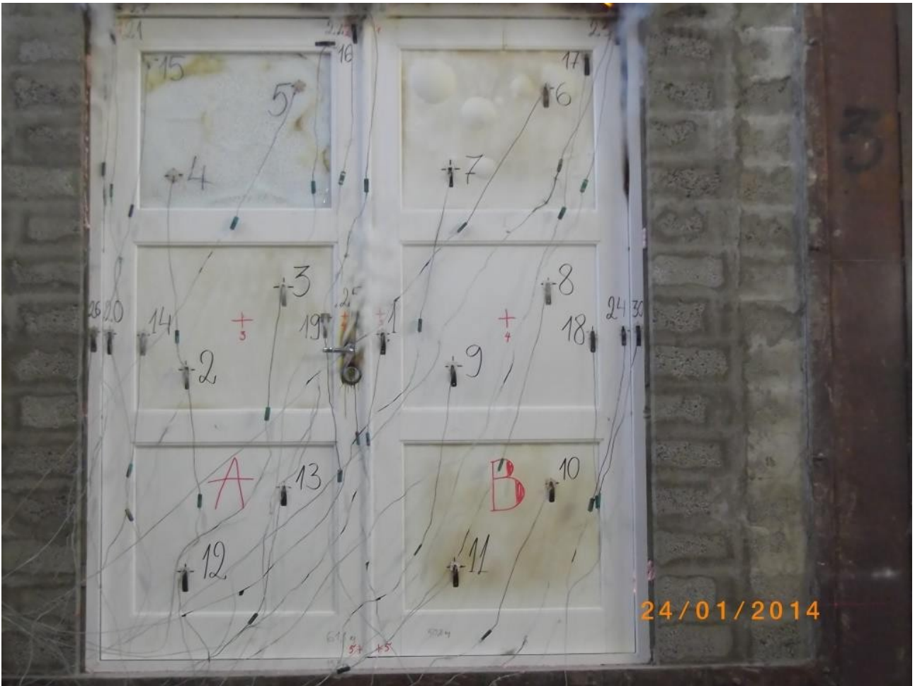
Photograph 10. View on the test specimen from unexposed side during the test (time: 32 minutes 05 seconds)
